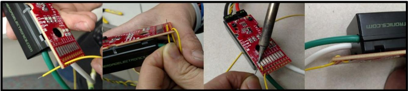
*Shown above is the process of soldering the wires onto the breakout board.*
