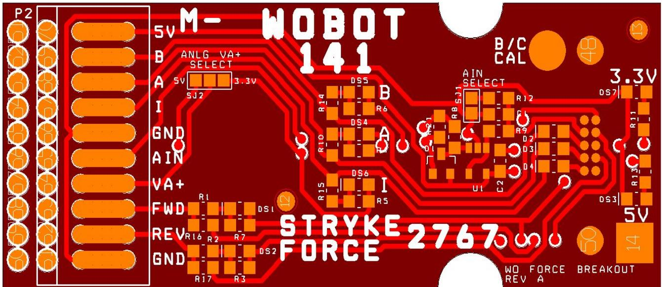
*Top View of the Sentinel Breakout Board, rev A*
