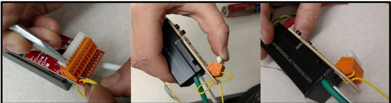
*Shown above is the process of wiring to the WAGO terminal strip.*
