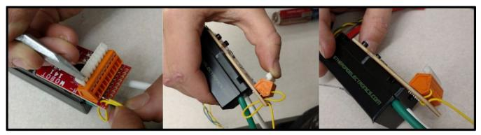
Shown above is the process of wiring to the WAGO terminal strip.
