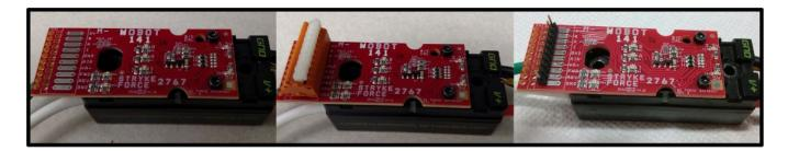
To the left, the basic the Sentinel Talon-SRX Breakout Board. The center view is of the Sentinel Talon-SRX Breakout Board shown with a WAGO 233-510 quick-release terminal block. To the right is the Sentinel shown with a header pin strip.
