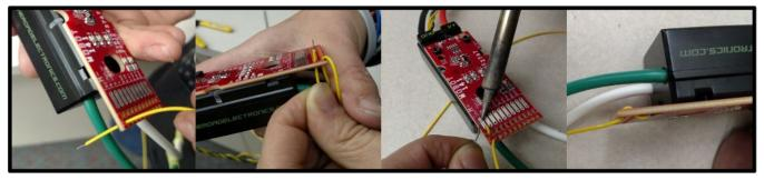
Shown above is the process of soldering the wires onto the breakout board.
